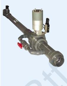
To safeguard the storage tank when using a compressed air feed from the feed tank, TECHAP offers its quick-acting fill protector as a complete unit (fast-closing valve including control unit, sensor and bypass valve with pipework) in nominal diameters DN 32, 40, 50, 65 and 80. There is a choice of the following materials: PVC, PP, VA (1.4571) and St.37.
