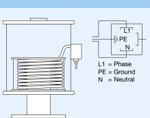
For binding agents BM1 and BM2, the heater should only be activated when there is a risk of frost. For BM4, the heater should always be activated.
